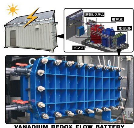
VANADIUM REDOX FLOW BATTERY
